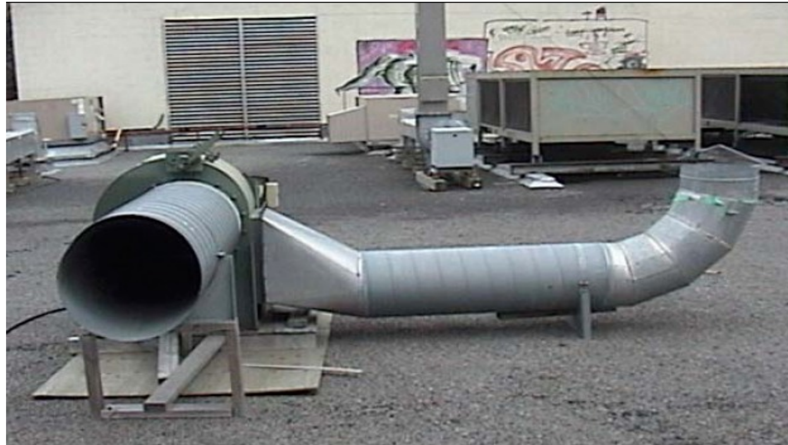
Photograph of the test stack used on the BE building (low stack with h_s=1\text{m} )
